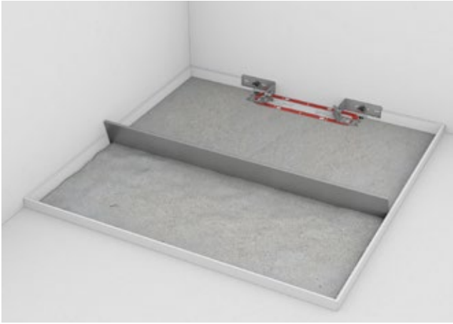
Step 3: The screed is installed with a gradient of 1 to 2% to the wall. The factory fitted bare-wall protection protects the drain from damage and dirt in the process.
