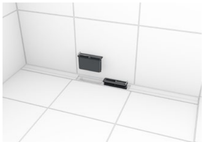
Step 8: The odour traps can also be easily removed for thorough cleaning of the shower profile.
