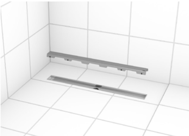
Step 6: After tiling and grouting, the cover is inserted into the channel body. This concludes the assembly. To enable thorough cleaning, the cover can also be removed any time after assembly and replaced again.
