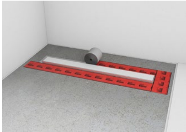
Step 3: The Seal System sealing tape is glued on in such a way that it overlaps with the shower channel flange and the screed.
