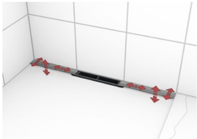
Step 6: The shower profile can still be finely adjusted both horizontally and vertically even after the drain is mounted in the screed and can be adjusted to different thicknesses of wall and floor covers.
