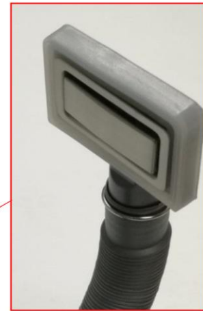
Replace rubber ring by silicone gasket
